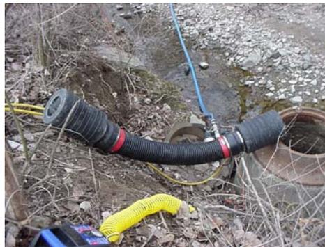
2. Fill the manhole to the top of casting and maintain this level for a period of at least 30 minutes. This is to allow exfiltration out of the manhole to fill the voids in the soil surrounding the manhole in dry periods in order to simulate a high groundwater condition.
